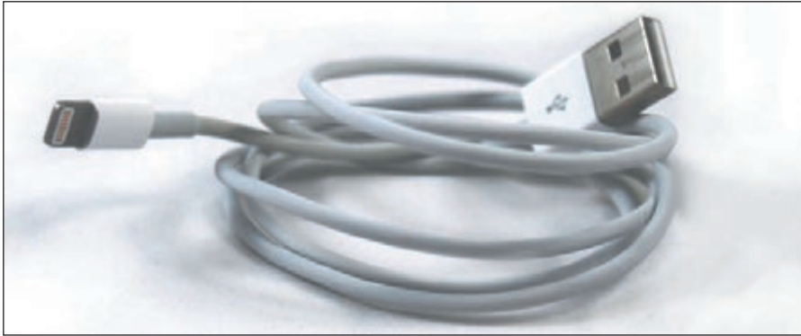
Figure 9-30 A Lightning cable by Apple, Inc., has a USB connector for the computer end and a Lightning connector for an iPhone or iPad
