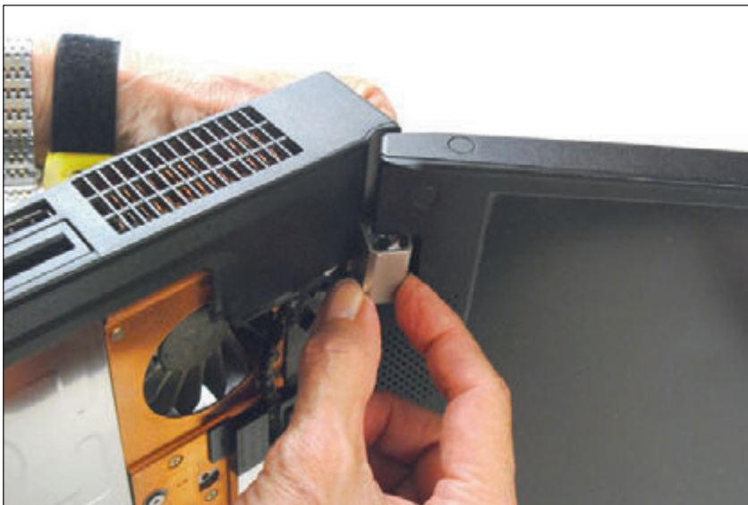
Figure 6-59 Remove the hinge cover from the laptop hinge
