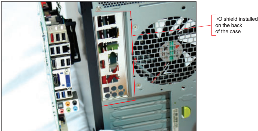
Figure 2-41 Make sure the holes in the I/O shield match up with the ports on the motherboard
