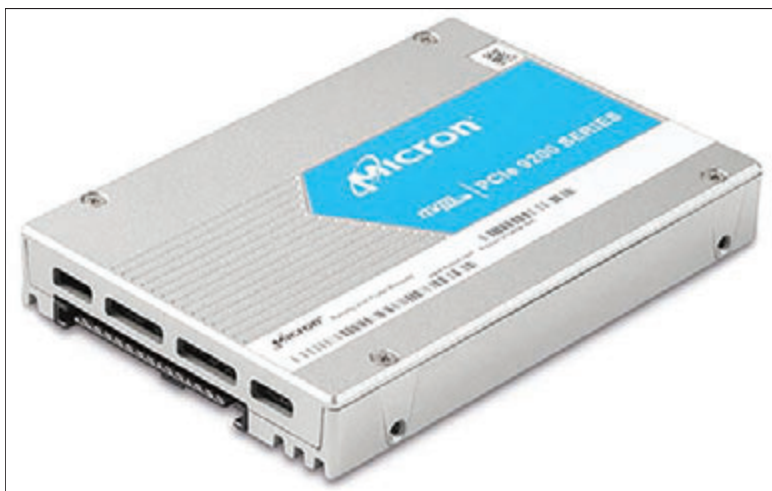
Figure 5-16 A U.2 2.5" SSD uses the NVMe and PCIe interface standards and connects to a U.2 port on the motherboard
