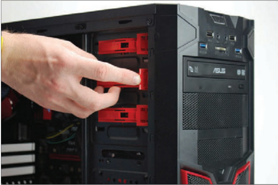
Figure 1-41 To remove this optical drive, first release the clip to release the drive from the bay
