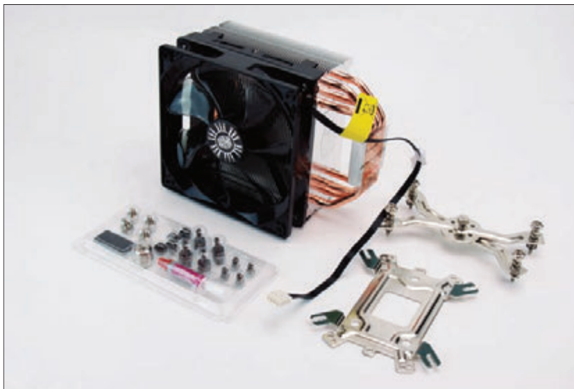
Figure 3-14 A heavy-duty cooler may have a strengthening plate, heat sink, fins, a fan, and several screws, nuts, and bolts
