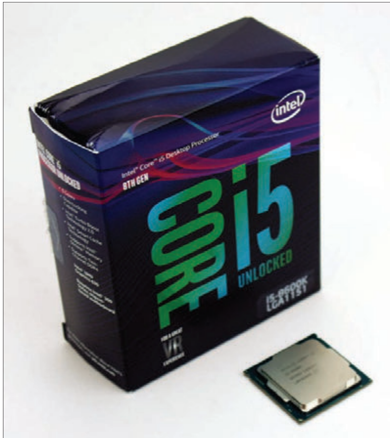
Figure 3-5 The Intel Core i5-8600K 14-nm, 3.60-GHz, 9-MB cache processor installs in the 8th generation LGA1151 socket
