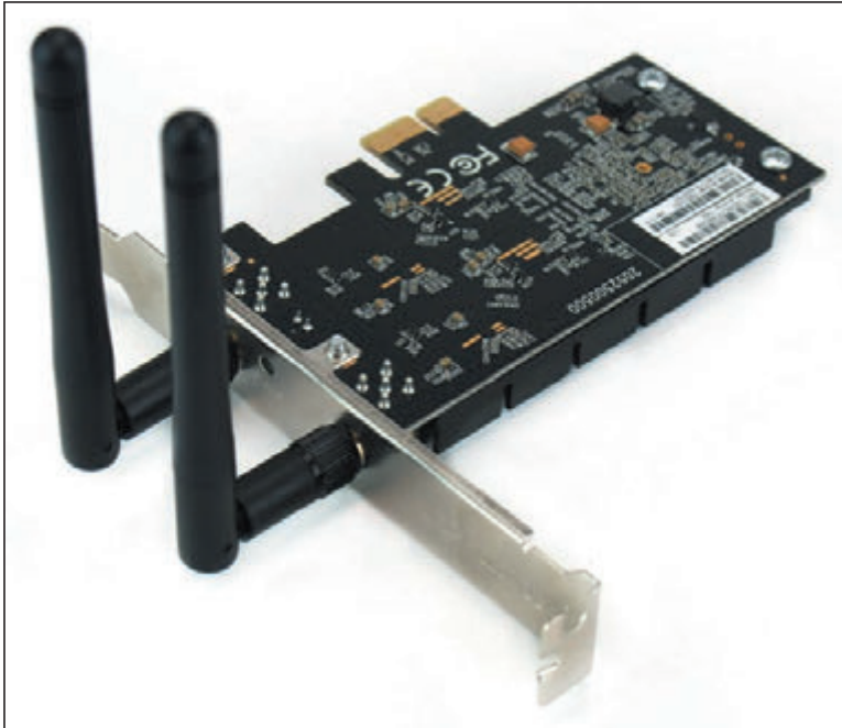
Figure 7-54 A wireless network adapter with two antennas supports 802.11a/b/g/n/ac Wi-Fi standards
