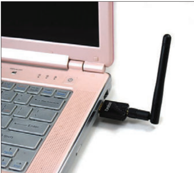
Figure 1-59 This USB to Wi-Fi adapter plugs into a USB port to connect to a local wireless network
