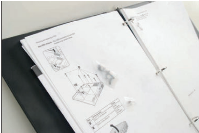
Figure 1-75 Tape screws beside the step in the manufacturer documentation that told you to remove the screw
