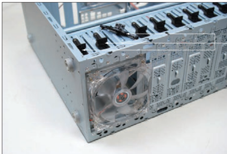
Figure 5-28 The removable bay has a fan in front and is anchored to the case with locking pins
