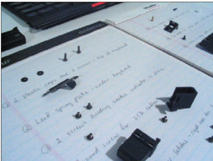
Figure 1-74 Using a notepad can help you organize screws so you know which screw goes where when reassembling
