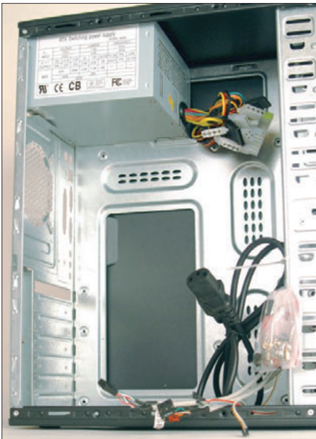
Figure 4-8 This case comes with a power supply, power cord, and bag of screws
