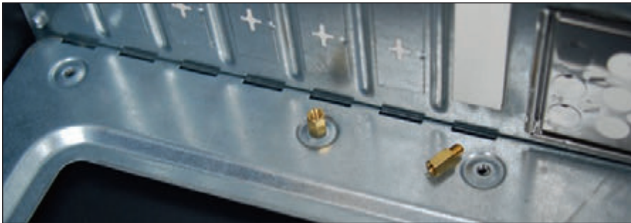
Figure 4-38 Spacers installed in case holes keep the motherboard from causing a short
