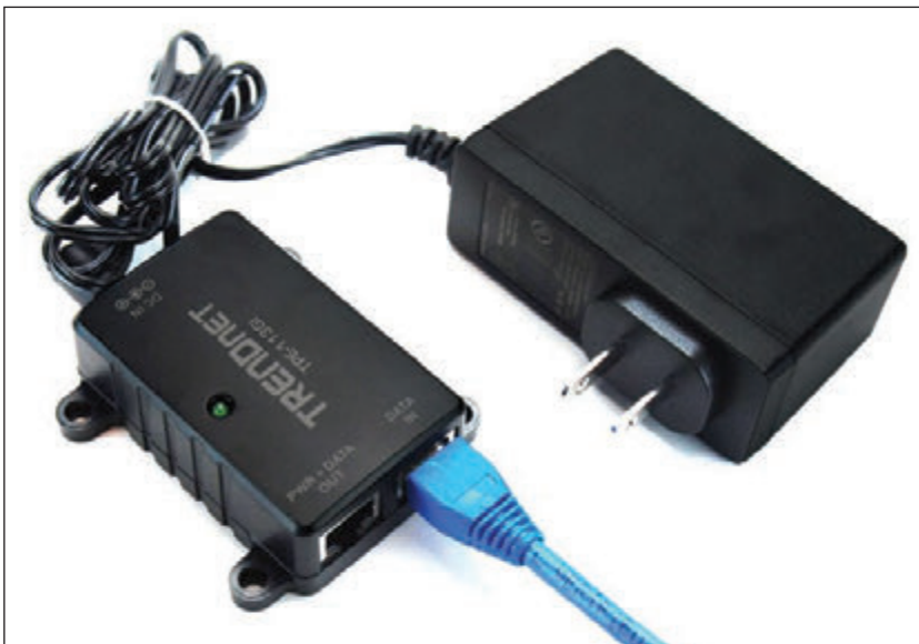
Figure 8-28 A PoE injector introduces power to an Ethernet cable
