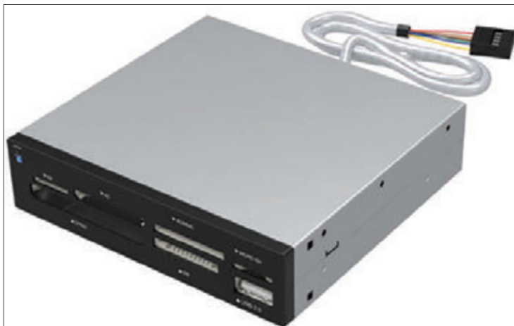
Figure 5-58 This 7-slot USB 2.0 Internal Memory Card Reader and Writer by Sabrent supports multiple types of smart cards
