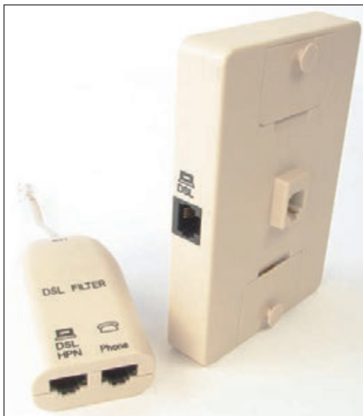
Figure 7-2 When DSL is used in your home, filters are needed on every phone jack except the one used by the DSL modem
