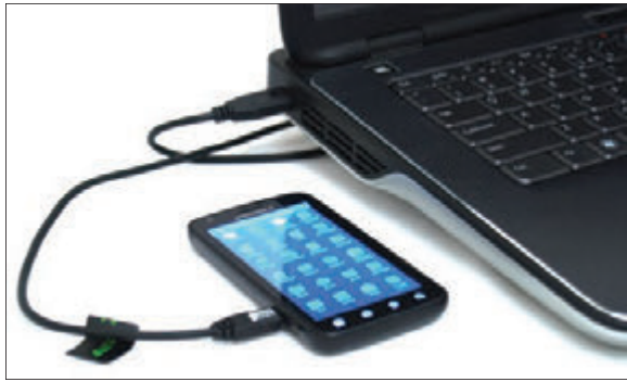
Figure 7-8 Tether your laptop to your cell phone using a USB cable
