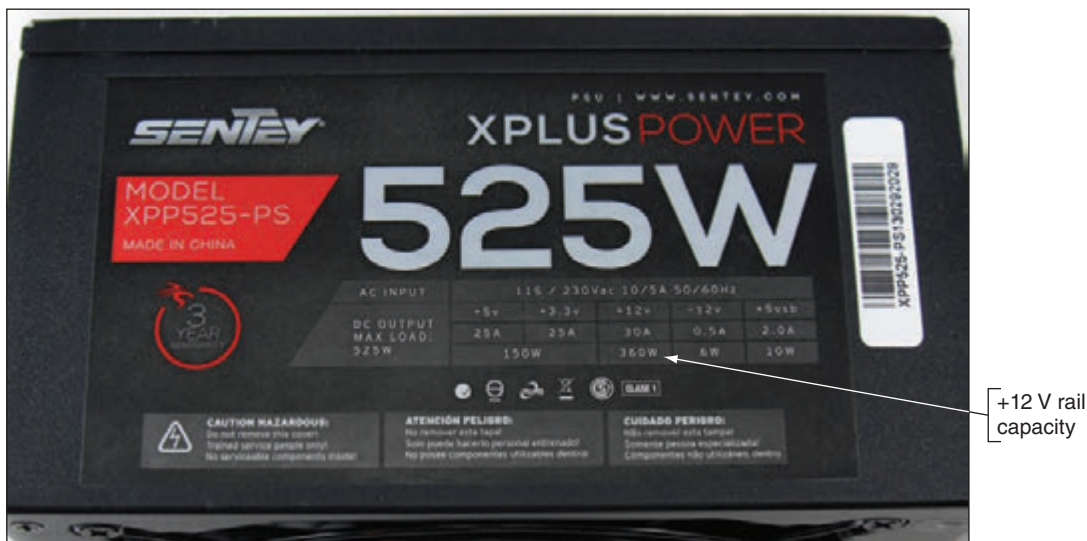
Figure 4-9 Consider the number and type of power connectors and the wattage ratings of a power supply
