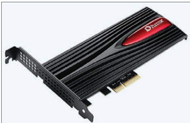
Figure 5-6 This SSD by Plexor is embedded on a PCIe ×4 version 3.0 expansion card and uses the NVMe interface standard
