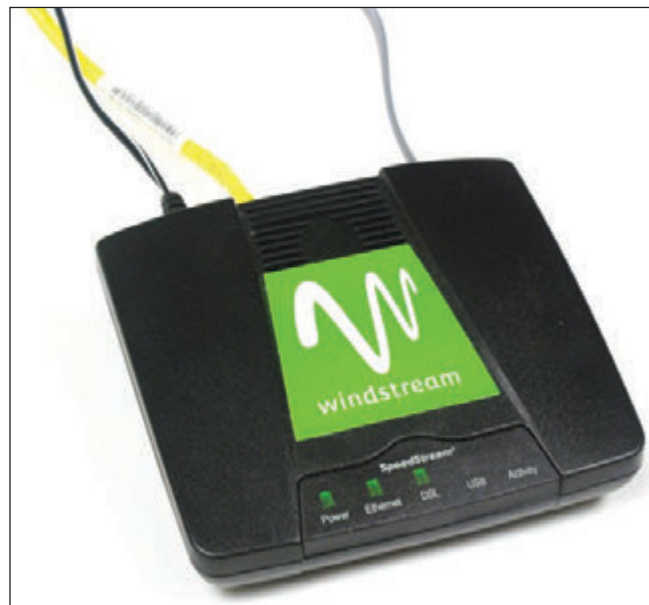
Figure 7-3 This DSL modem connects to a phone jack and a computer or router to provide a broadband connection to an ISP
