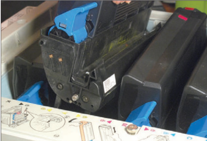
Figure 10-44 Remove the image drum and toner cartridge as one unit
