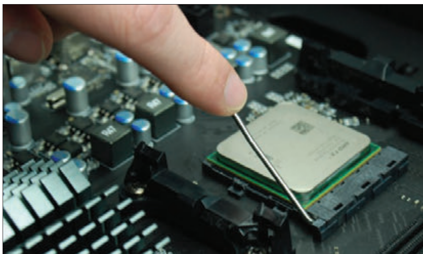
Figure 3-22 Lower the lever into place, which puts pressure on the processor
