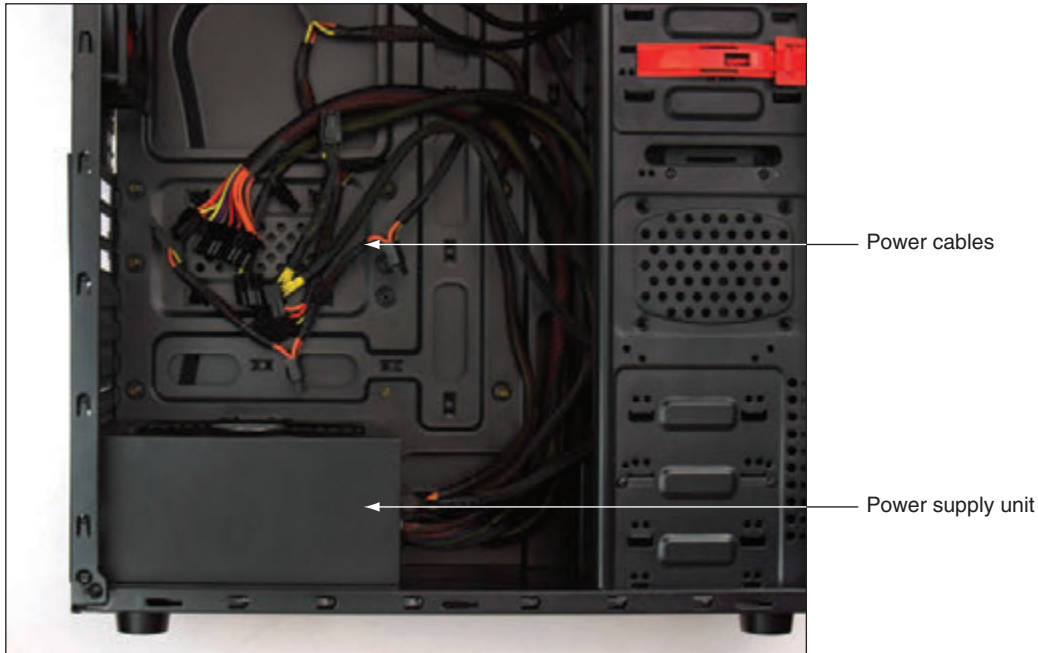
Figure 1-18 A power supply with attached power cables
