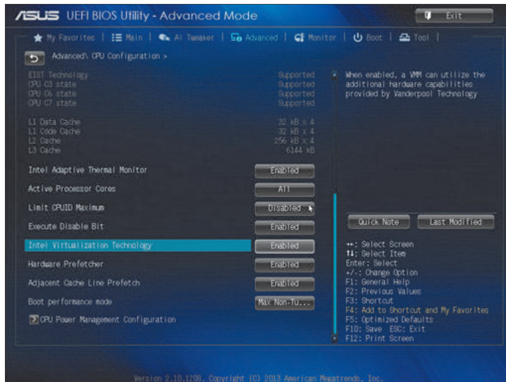
Figure 10-3 A UEFI setup screen to enable hardware virtualization
