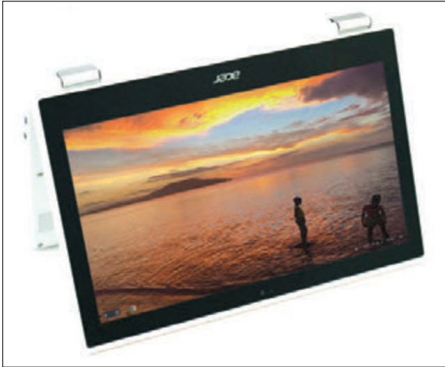
Figure 9-18 A Chromebook can be a lightweight laptop, a tablet, or a hybrid laptop-tablet
