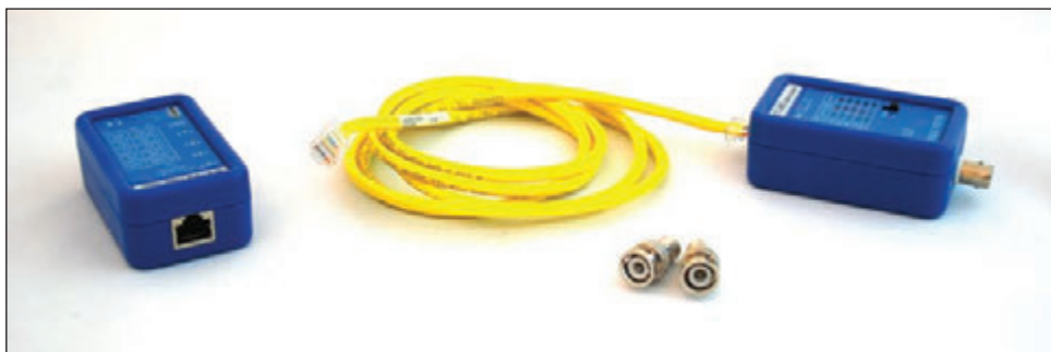
Figure 8-32 Use a cable tester pair to determine the type of cable and/or if the cable is good
