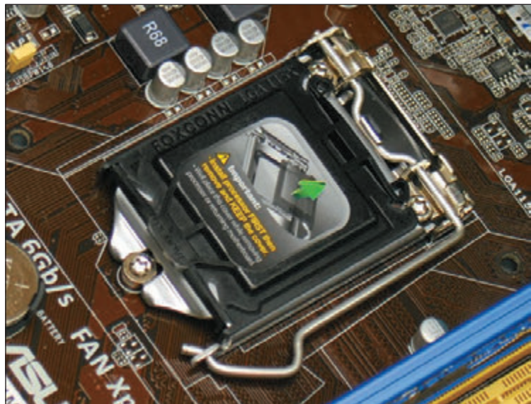
Figure 2-7 The LGA1150 socket with the protective cover installed
