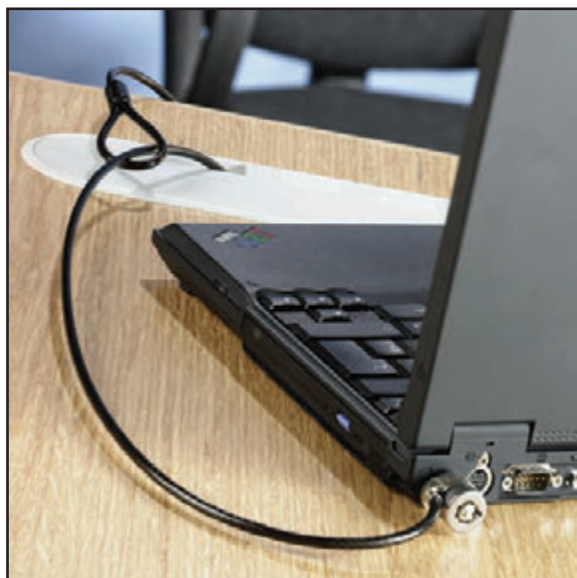
Figure 1-57 Use a cable lock system to secure a notebook computer to a desk to help prevent it from being stolen
