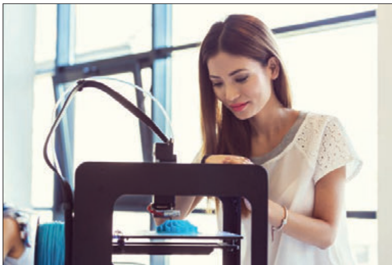
Figure 10-19 A 3D printer heats a plastic filament and layers the plastic to build three-dimensional objects
