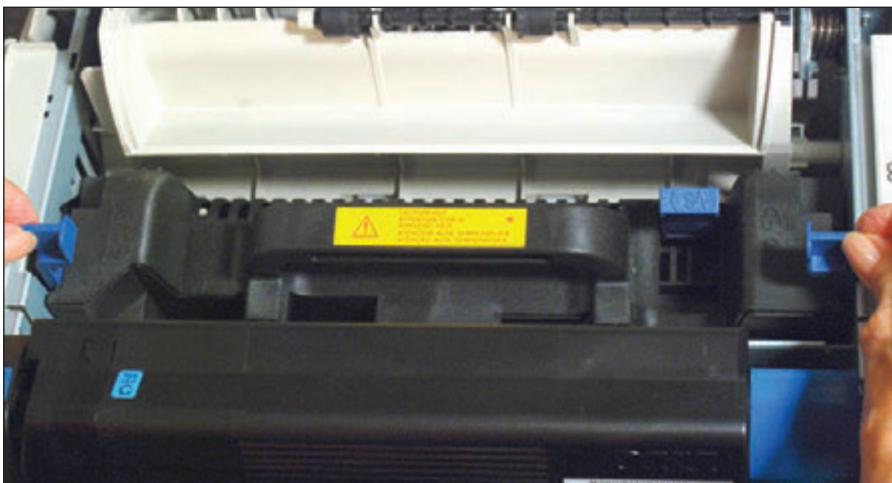
Figure 10-45 Pull the two fuser levers forward to release the fuser
