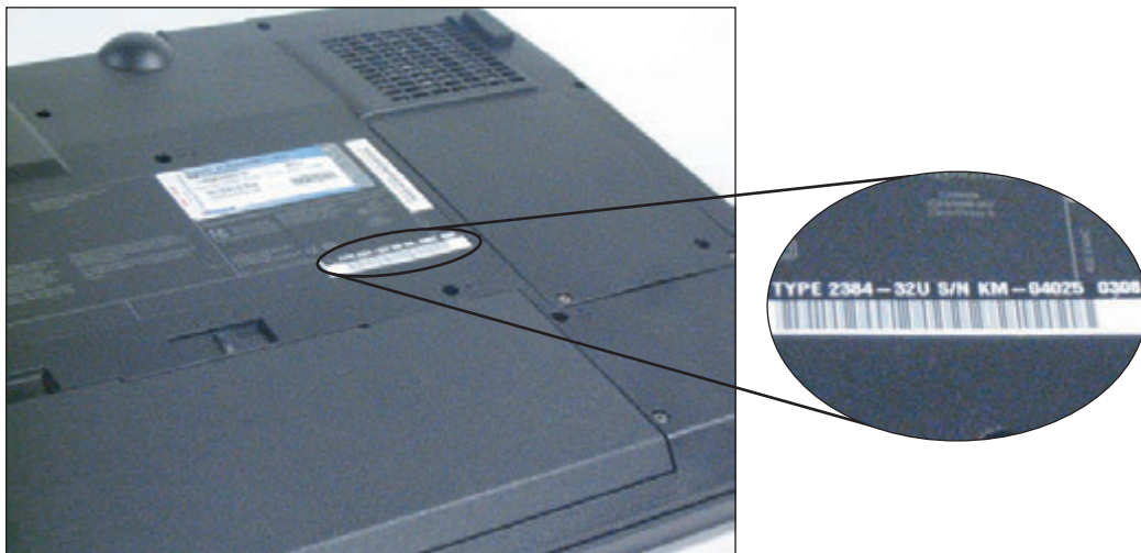
Figure 1-67 The model and serial number stamped on the bottom of a laptop are used to identify the laptop to service desk personnel
