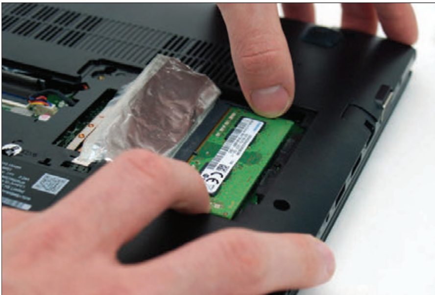
Figure 1-81 Release the latches on both edges of the socket to remove the memory modules
