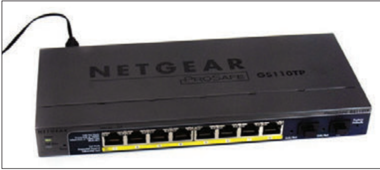
Figure 8-19 This Gigabit Ethernet switch by NETGEAR has eight Ethernet ports
