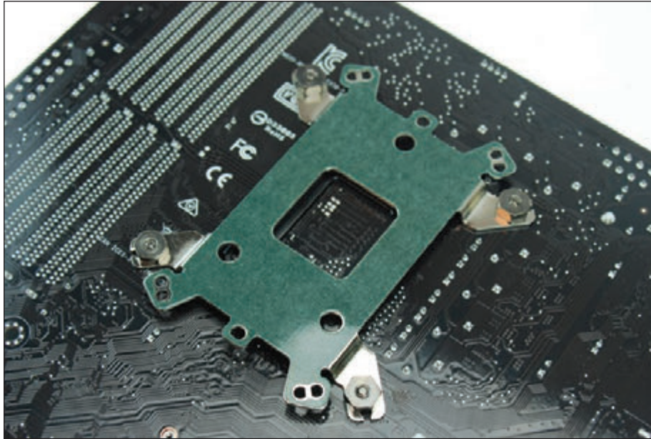
Figure 3-16 A cooler assembly plate on the bottom of the motherboard prevents a heavy cooler from bending the board
