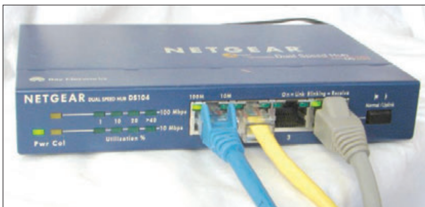
Figure 8-18 This hub supports 10-Mbps and 100-Mbps Ethernet speeds
