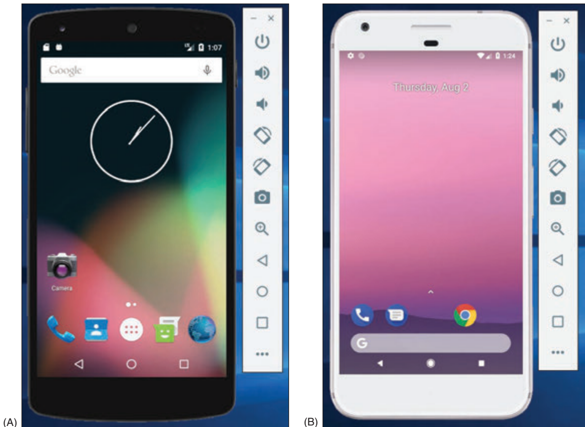
Figure 9-69 (A) An emulated Nexus 5 with Android Marshmallow, and (B) an emulated Pixel XL with Android Oreo
