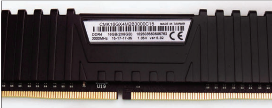
Figure 3-42 Look for imprinted information about a DIMM
