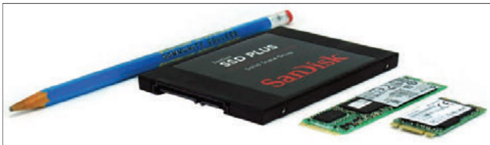
Figure 5-5 Solid-state drives in two form factors: 2.5" SSD and two lengths of M.2 SSD cards
