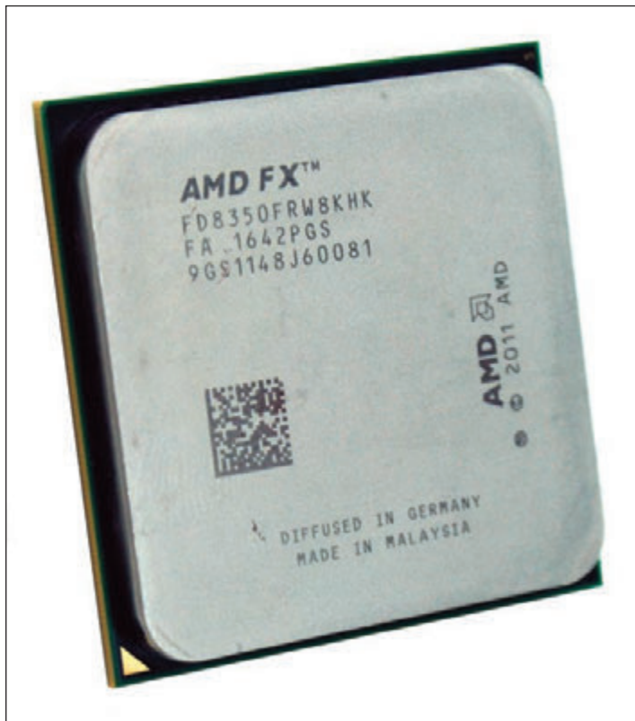
Figure 3-6 The AMD FX processor installs in the AMD AM3+ socket and has eight cores
