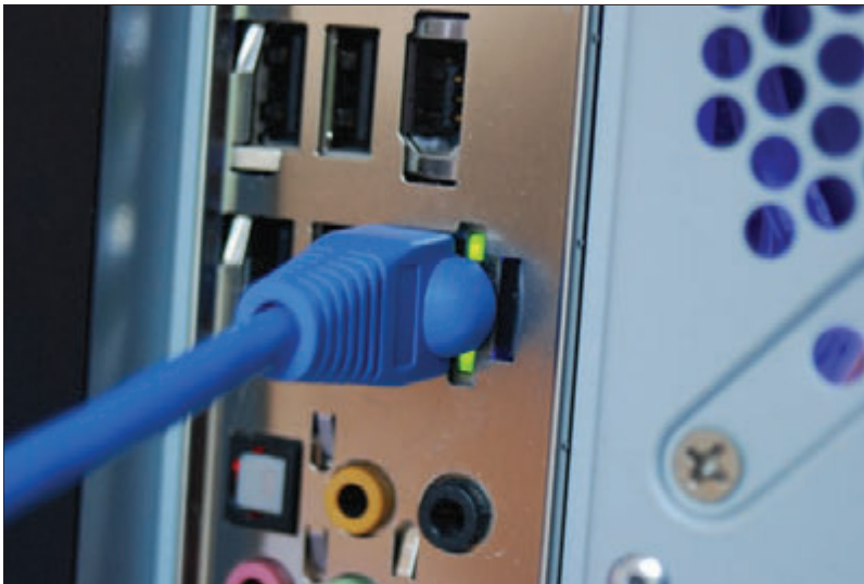
Figure 8-52 Status indicator lights verify connectivity for a network port
