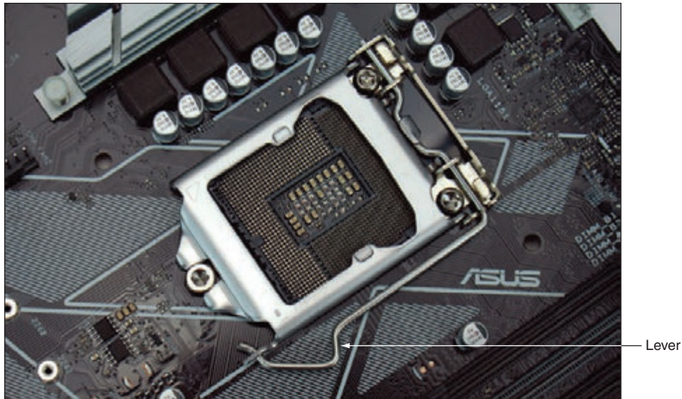
Figure 3-9 The exposed socket is extremely delicate
