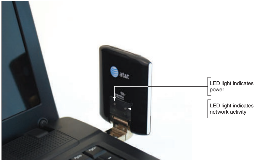
Figure 1-60 This USB device by Sierra Wireless provides a wireless connection to a cellular network
