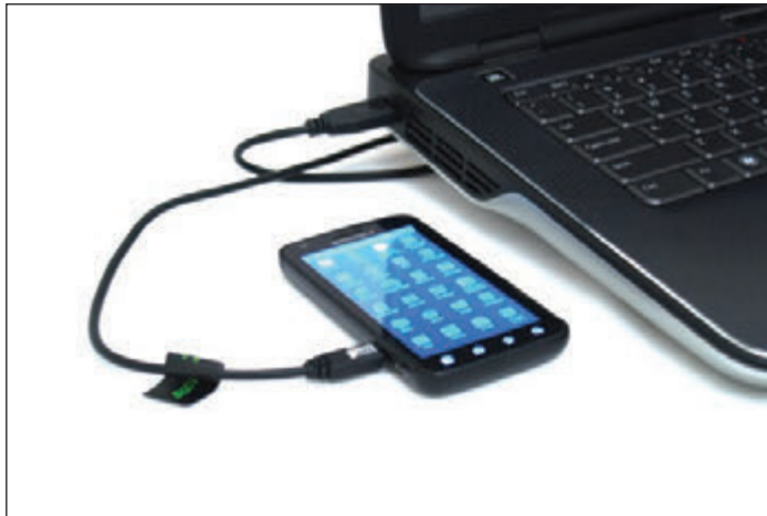
Figure 9-24 Tether your smartphone to your laptop using a USB cable
