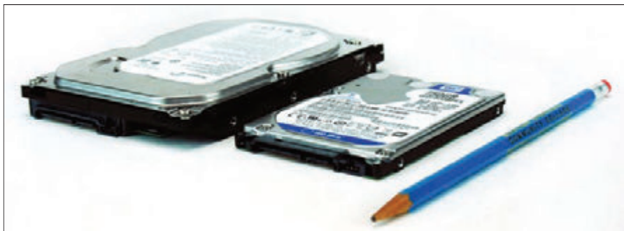
Figure 5-3 A magnetic hard drive for a desktop is larger than that used in laptops
