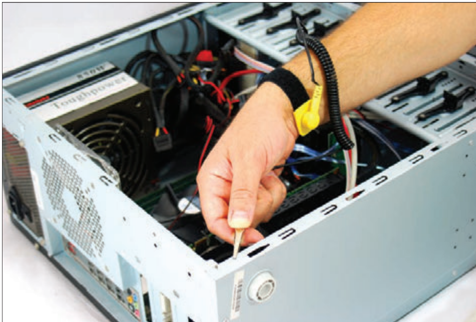
Figure 1-11 Attach the alligator clip of your ground bracelet to the side of the computer case
