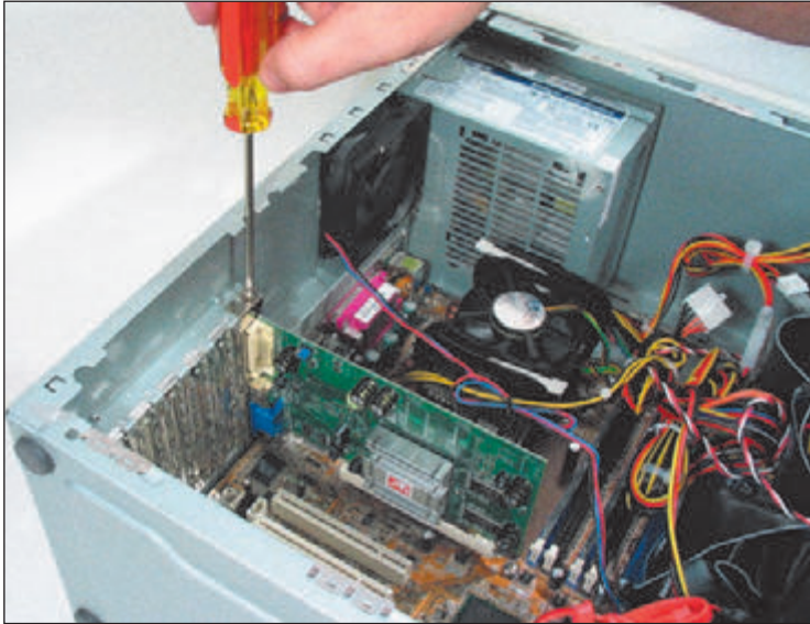
Figure 6-33 Secure the card to the case with a single screw
