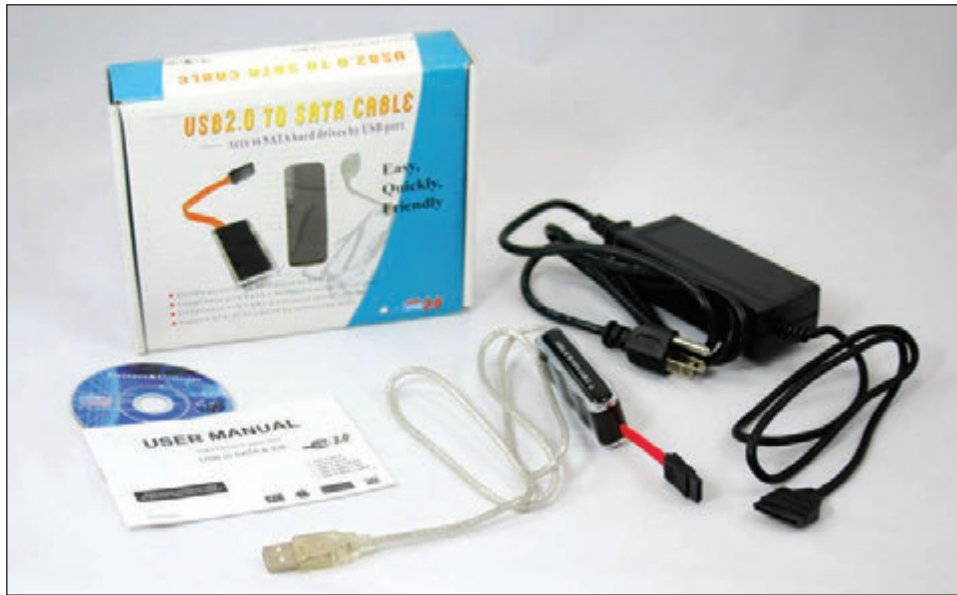
Figure 4-14 Use a USB-to-SATA converter to recover data from a drive that has a SATA connector
