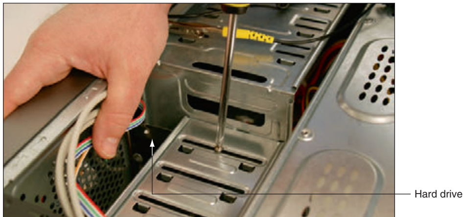
Figure 5-23 Secure the other side of the drive with one or two screws
