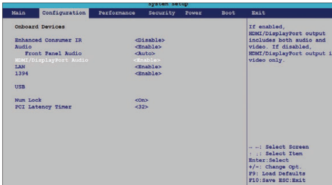
Figure 6-6 Use BIOS/UEFI setup to enable or disable onboard ports
