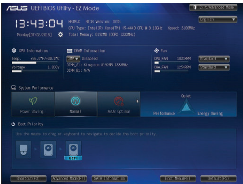
Figure 2-27 Information about the system is reported when you first access BIOS/UEFI setup
