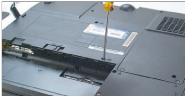
Figure 6-18 Remove screws on the bottom of the laptop
