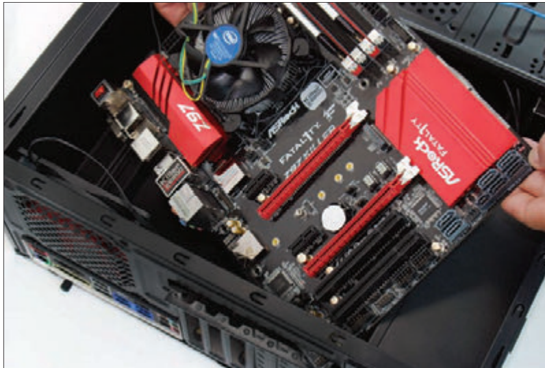
Figure 2-42 A motherboard with processor, cooler, and memory modules installed is ready to go in the case
