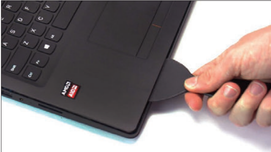
Figure 1-84 Using a spudger helps prevent harming the casing when prying it open
