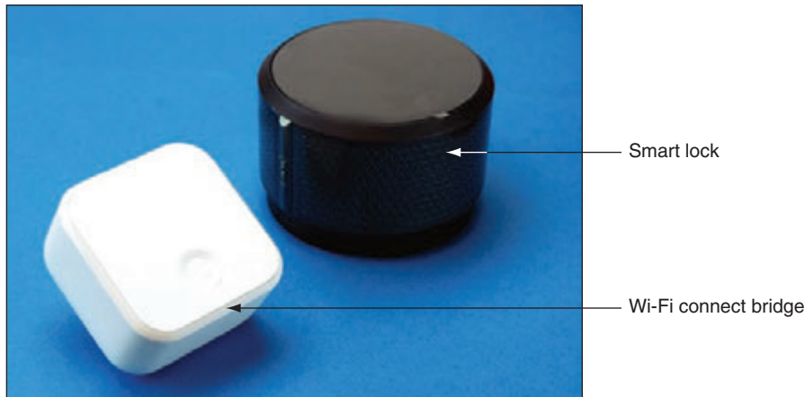
Figure 9-51 The August Smart Lock Pro automatically unlocks or locks as the user's Bluetooth-enabled smartphone moves closer or farther away
