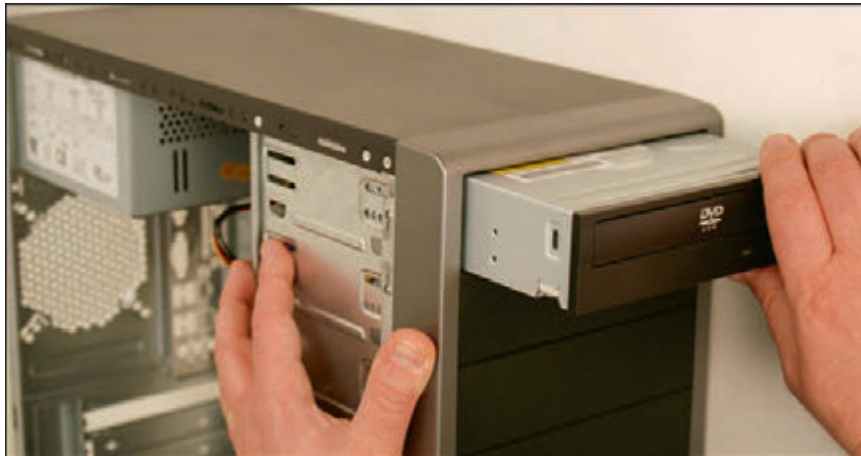
Figure 5-52 Slide the drive into the bay flush with the front panel
