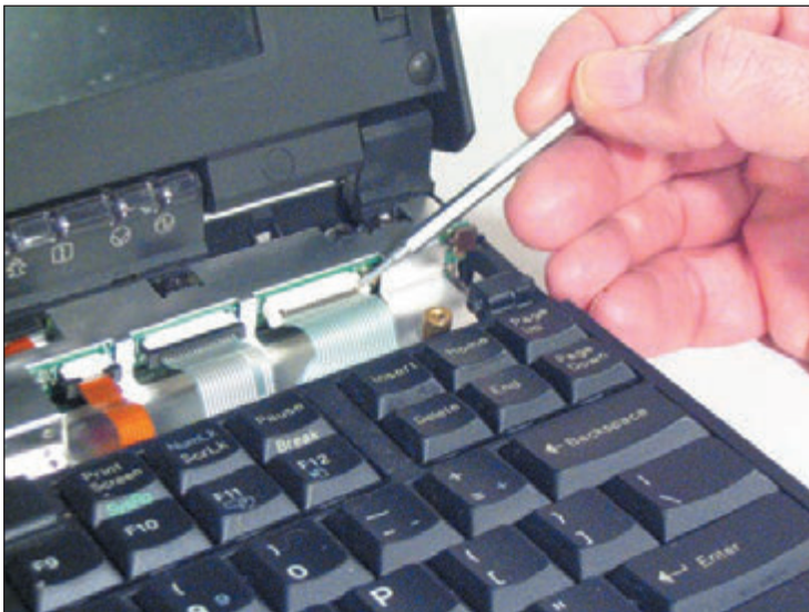
Figure 1-77 Three ZIF connectors hold the three keyboard cables in place
