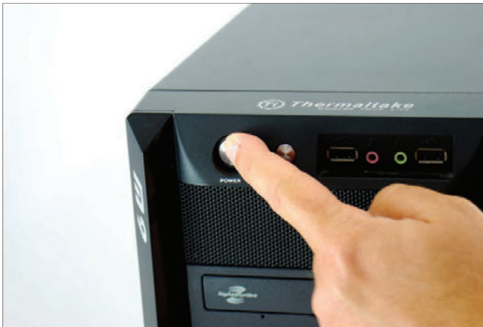
Figure 1-6 Press the power button after the computer is unplugged
