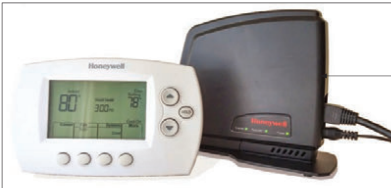
Figure 9-56 Use your phone, an Echo Dot, or a Google Home smart speaker to control this wireless thermostat
