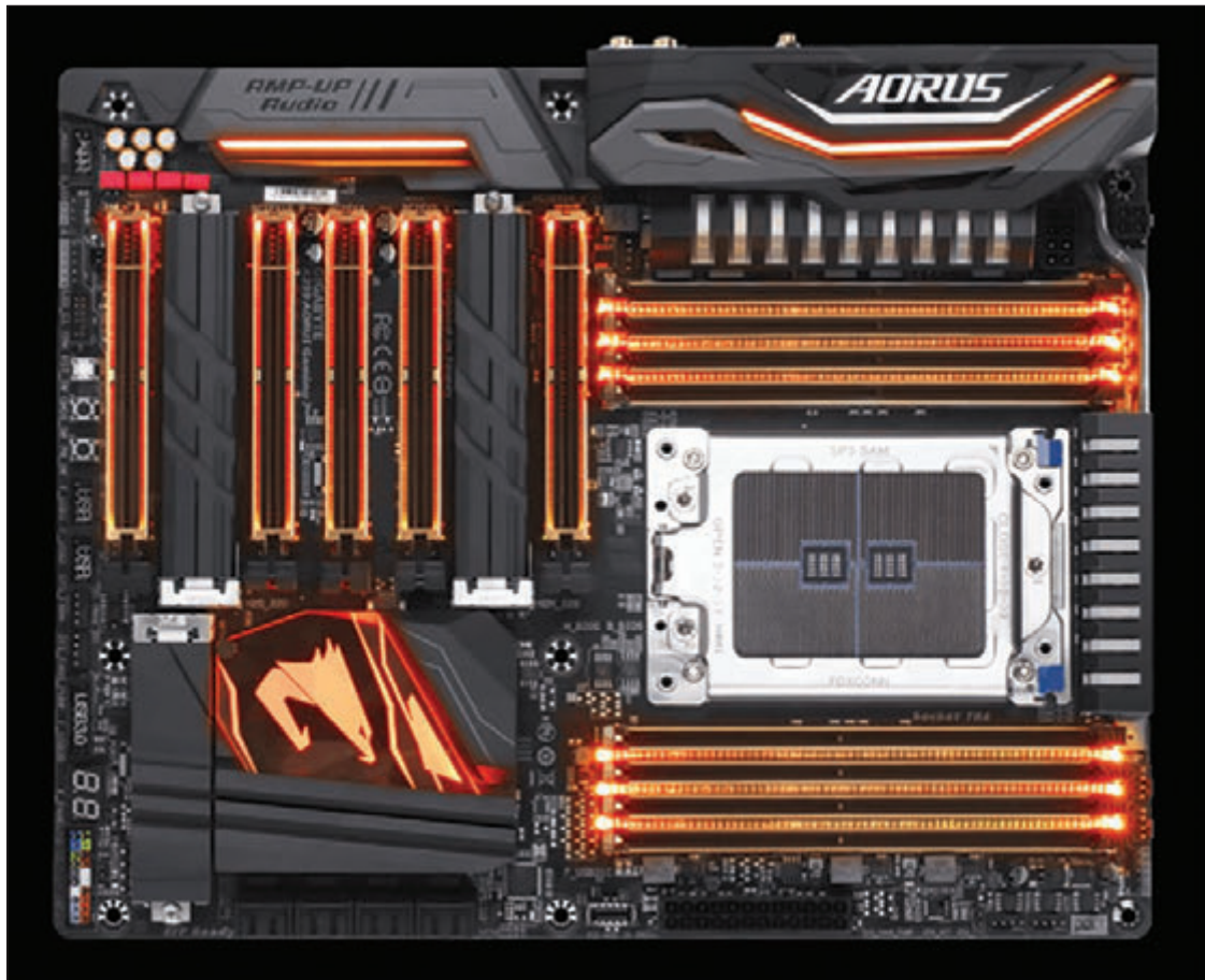
Figure 3-35 The Gigabyte AMD X399 Gaming motherboard has eight DIMM DDR4 slots and supports quad channeling
