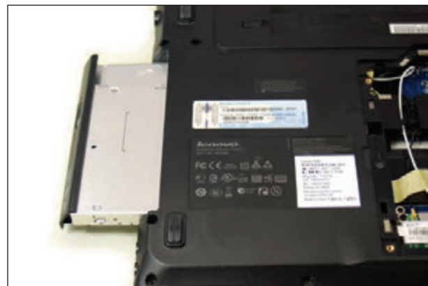
Figure 5-56 Push the optical drive out the side of the case
