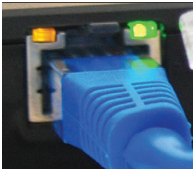
Figure 7-30 Status indicator lights for the onboard network port
