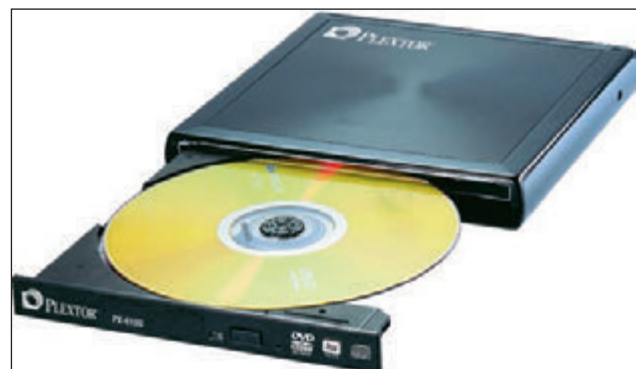
Figure 5-49 The PX-610U external DVD±RW drive by Plextor uses a USB 2.0 port
