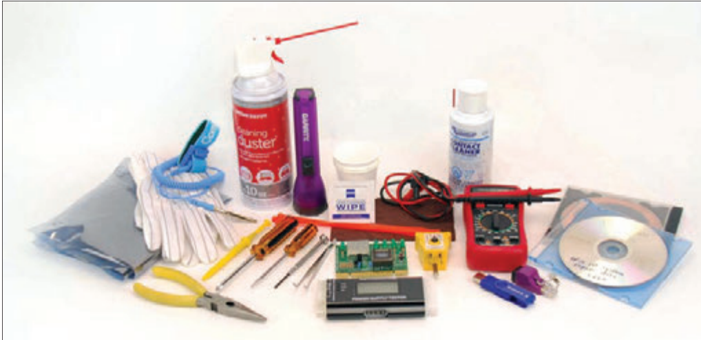
Figure 1-1 Tools used by IT support technicians when maintaining, repairing, or upgrading computers
