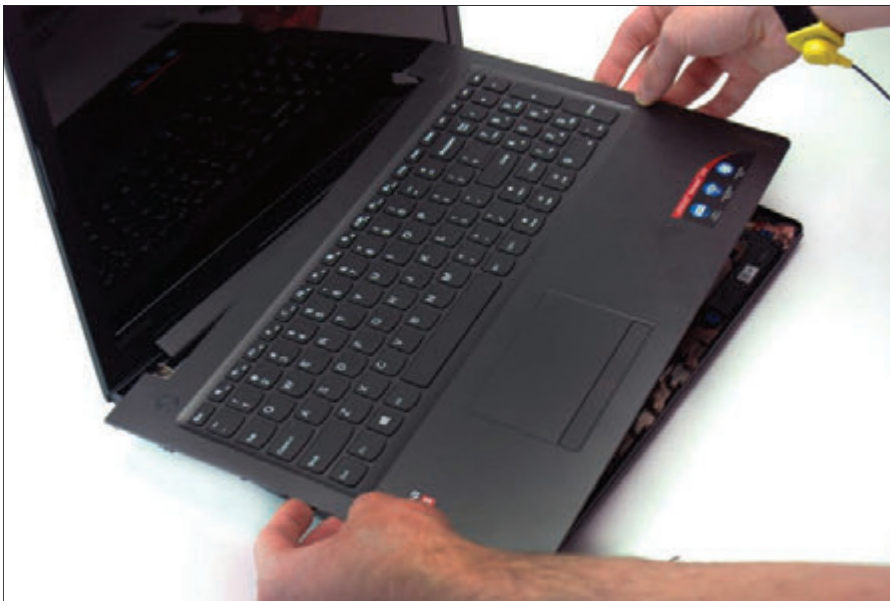
Figure 1-85 Disconnect both the touch pad board cable and the keyboard cable to remove the keyboard
