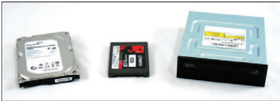
Figure 1-17 Two types of hard drives (larger magnetic drive and smaller solid-state drive) and a DVD drive
