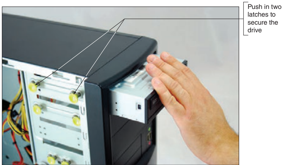
Figure 1-45 Align the front of the drive flush with the case front and then anchor with a screw
