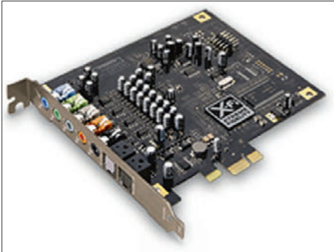
Figure 6-36 The Sound Blaster X-Fi Titanium sound card by Creative uses a PCIe \times 1 slot
