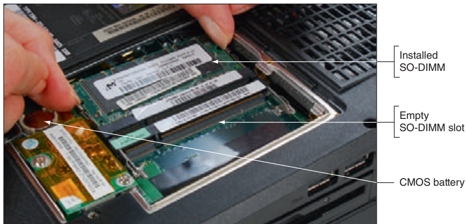
Figure 3-49 Pull apart the clips on the memory slot to release the SO-DIMM
