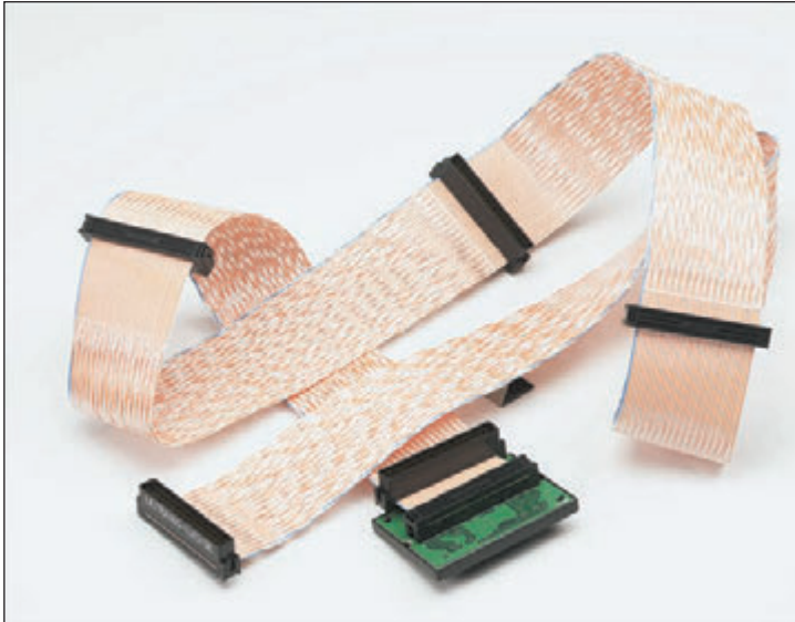
Figure 5-10 This 68-pin internal SCSI ribbon cable can connect several SCSI devices
