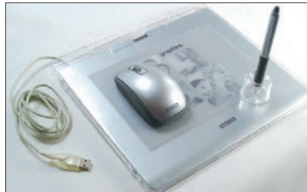
Figure 6-28 A graphics tablet and stylus are used to digitize a hand drawing
