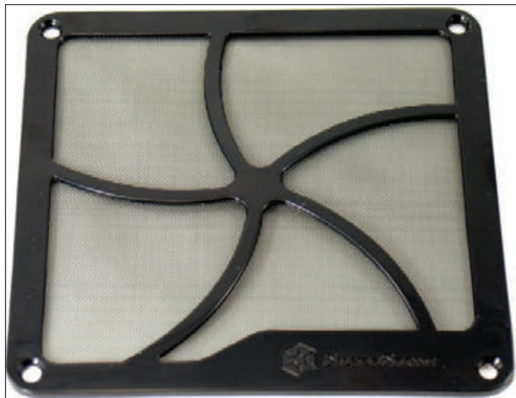
Figure A-10 This air filter is designed to fit over a case fan, power supply fan, or panel vent on the case
