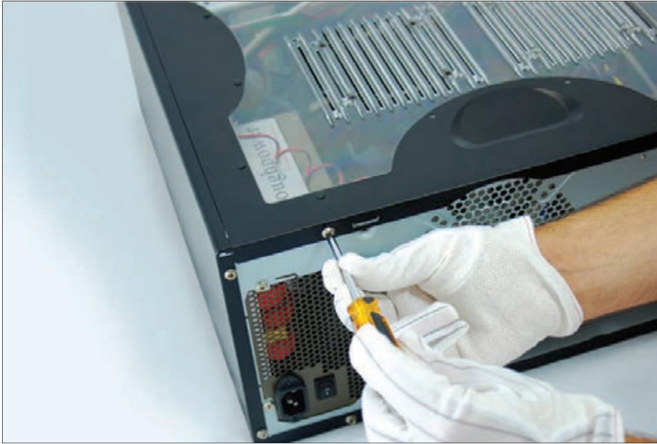
Figure 1-8 Locate the screws that hold the side panel in place
