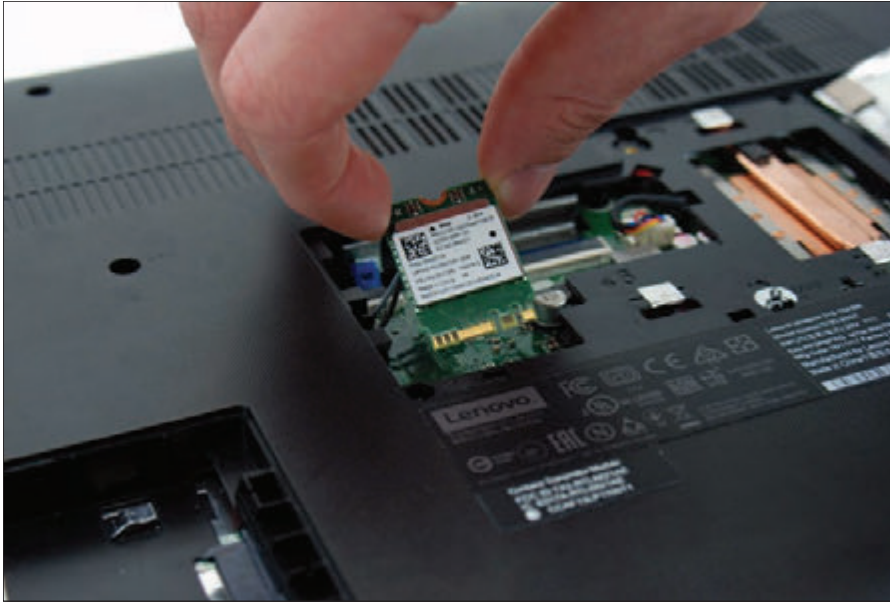
Figure 1-82 Pull the wireless card directly away from the socket to prevent damage to the card and socket
