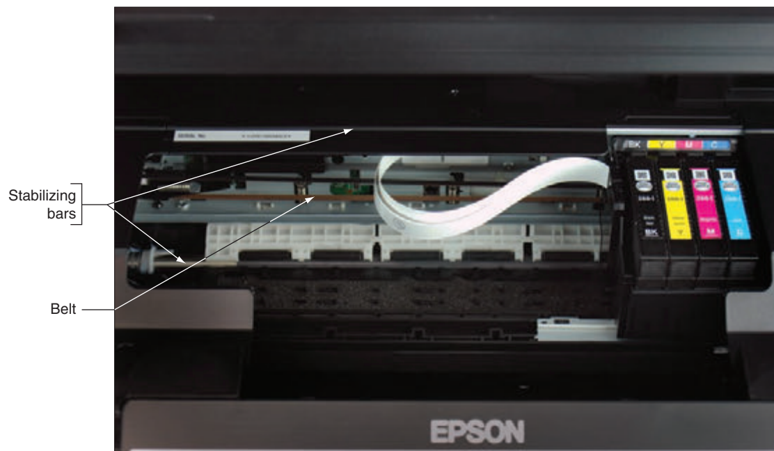
Figure 10-15 The belt and stabilizing bars used to move the print head across the page
