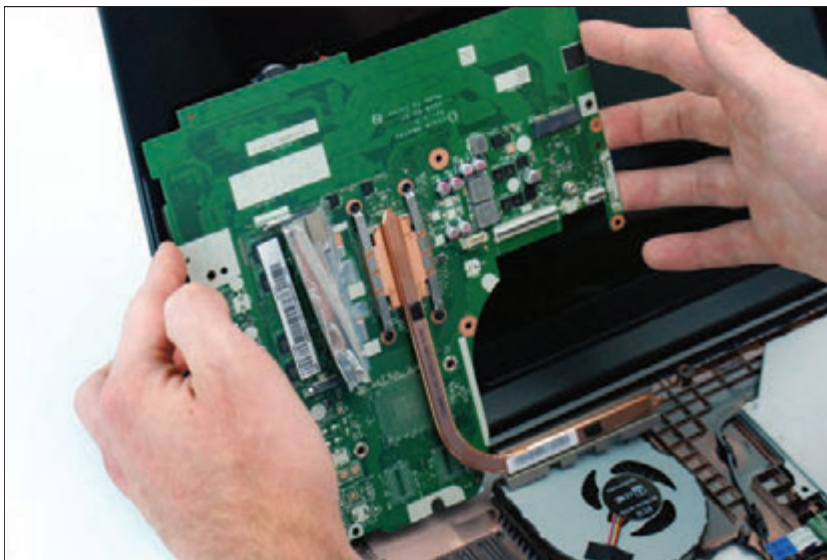
Figure 2-46 Disconnect the fan cable and screws holding the fan assembly to the system board
