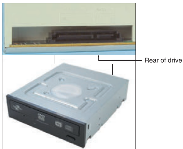
Figure 5-48 This internal DVD drive uses a SATA connection
