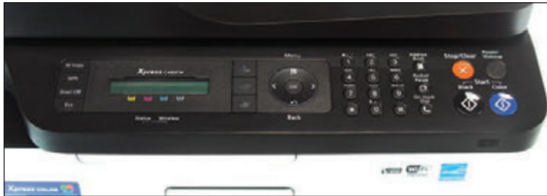
Figure 10-37 Use buttons on the front of the printer to display information, including the page count
