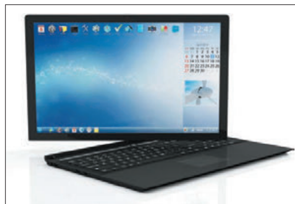
Figure 1-55 A laptop with a rotating display can do double-duty as a tablet computer
