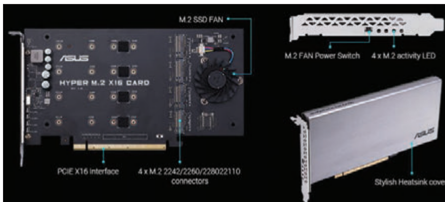
Figure 5-18 Install up to four M.2 SSDs in a bootable RAID array on this adapter card by Asus
