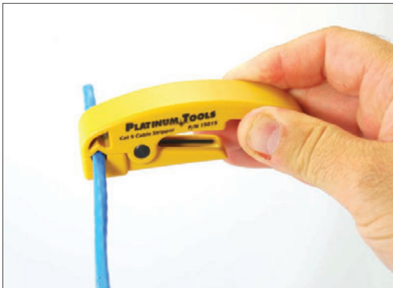
Figure 8-44 Rotate a wire stripper around the jacket to score it so you can slide it off the wire
