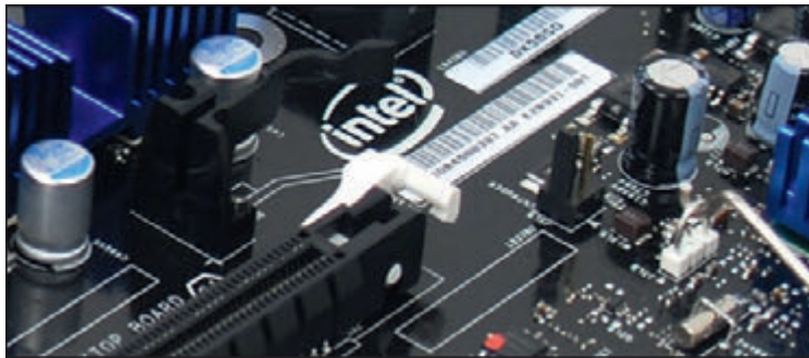
Figure 6-31 A white retention mechanism on a PCIe \times 16 slot pops into place to help stabilize a heavy video card
