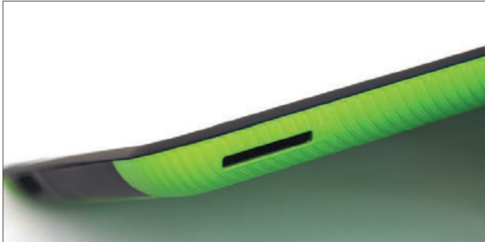
Figure 9-27 An Android device might provide a memory card slot to allow for extra storage
