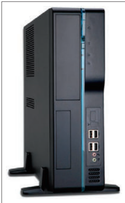
Figure 1-4 This slimline tower case supports a microATX motherboard
