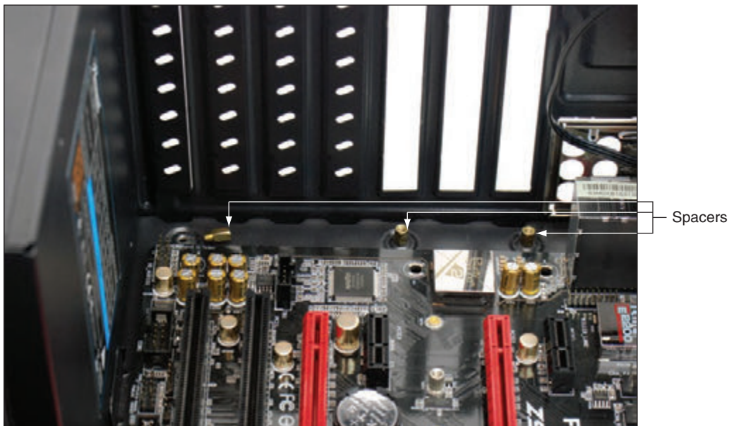
Figure 1-32 This motherboard connects to a case using screws and spacers that keep the board from touching the case
