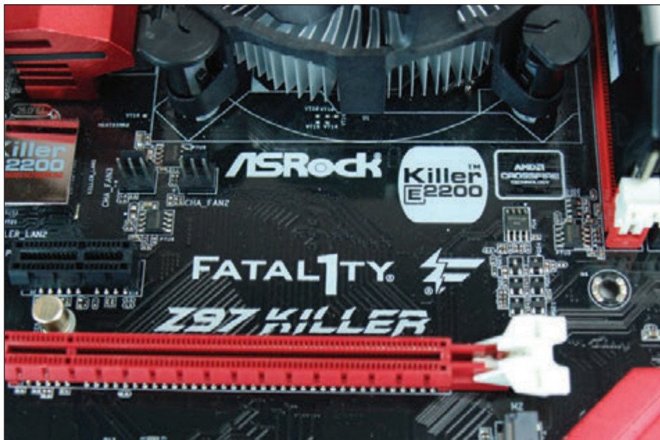
Figure 2-25 The motherboard brand and model are imprinted somewhere on the board
