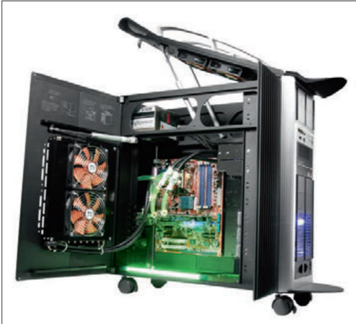
Figure 4-7 A liquid cooling system pumps liquid outside and away from components where fans can then cool the liquid
