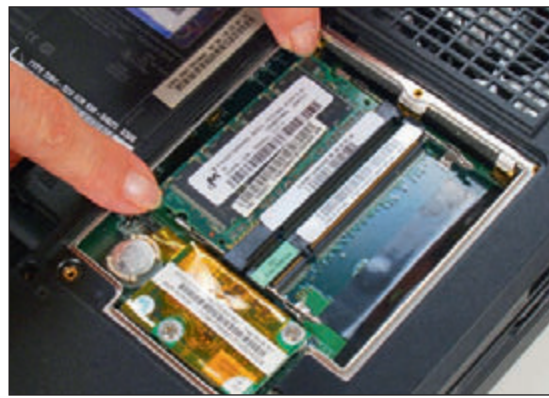
Figure 3-51 Push down on the SO-DIMM until it pops into the clips
