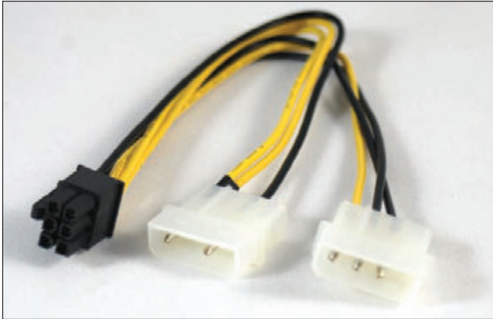
Figure 4-10 This adapter converts two Molex cables to a single 12-V 6-pin PCIe connector
