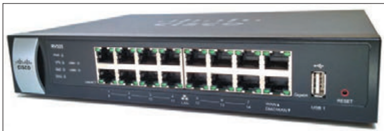
Figure 7-34 A router connects the local network to the Internet
