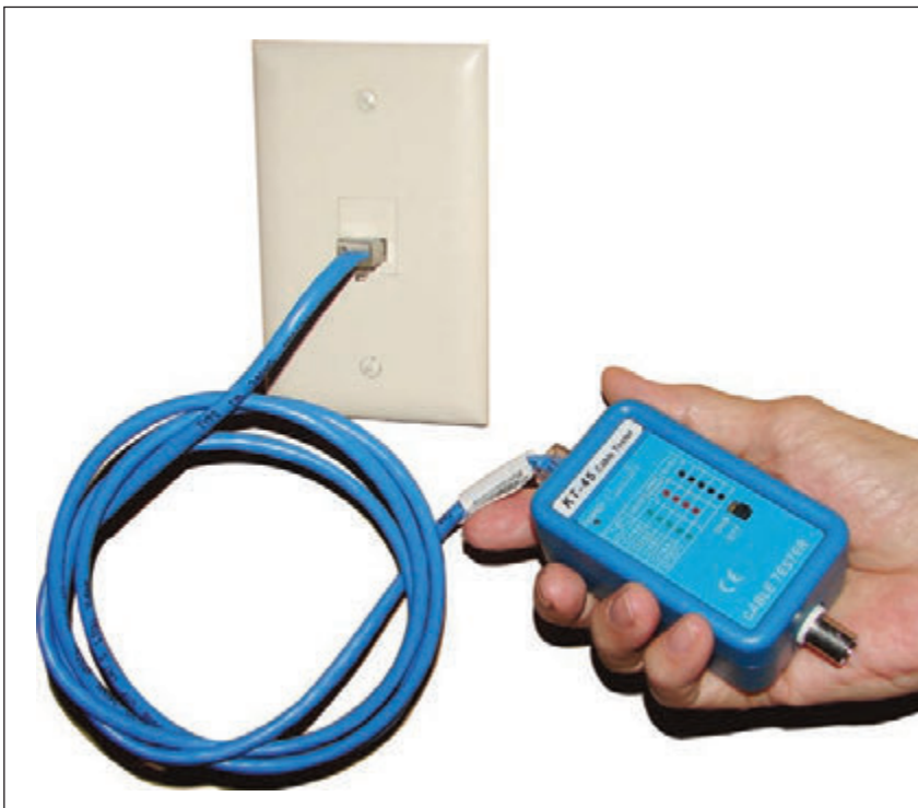
Figure 8-34 Use cable testers to find the two ends of a network cable in a building
