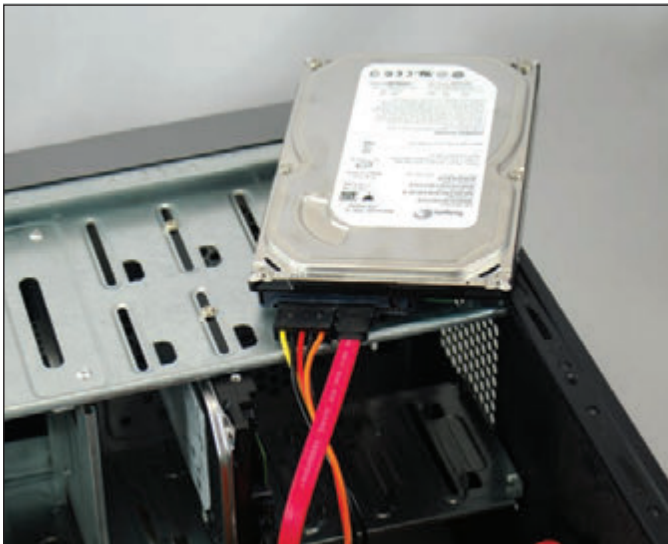
Figure 4-13 Move a hard drive to a working computer to recover data on the drive
