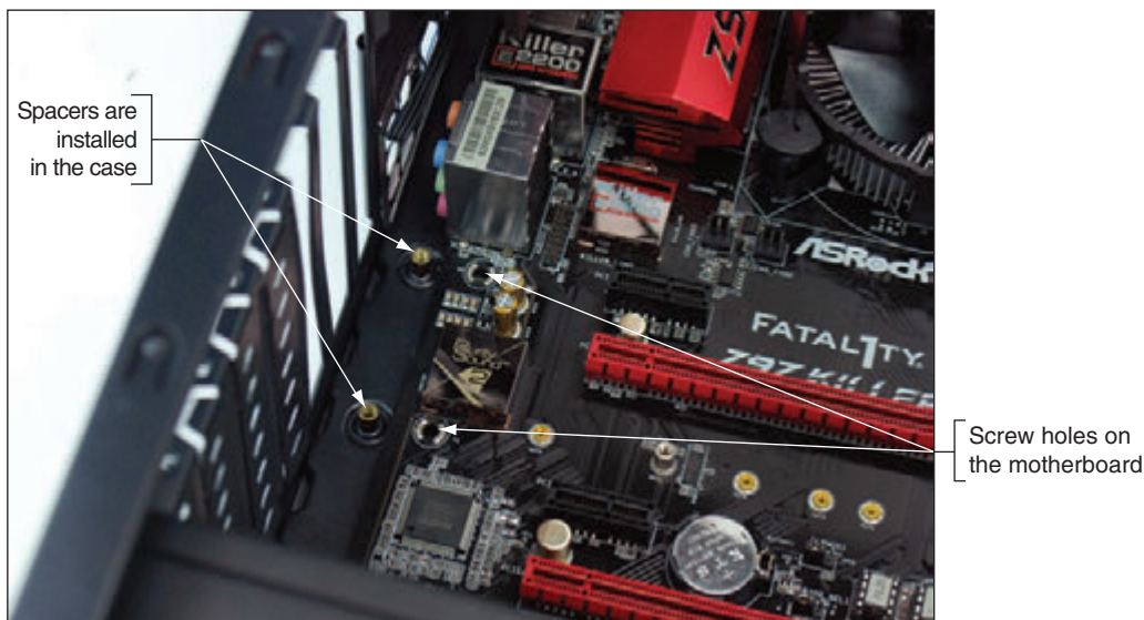
Figure 1-46 Align screw holes in the case with those on the motherboard
