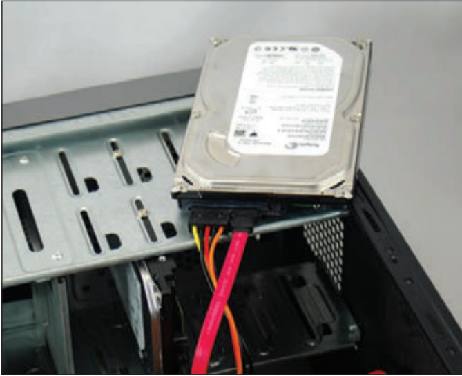
Figure 5-63 Temporarily connect a faulty hard drive to another system to diagnose the problem and try to recover data
