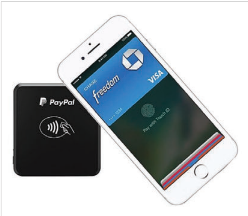
Figure 6-23 A tap pay device receives a transaction from a customer smartphone via NFC communication
