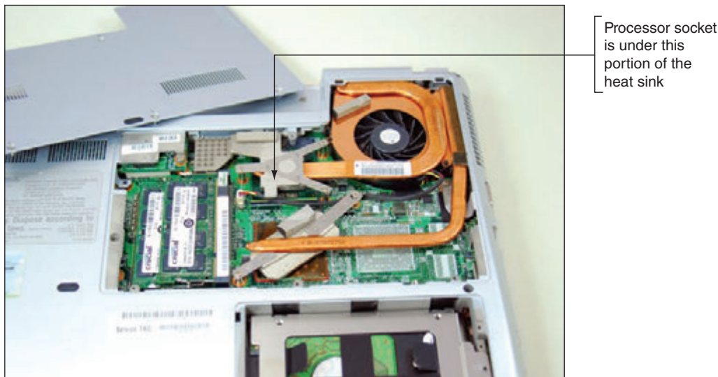
Figure 3-27 Remove the cover from the bottom of the laptop to expose the heat sink and fan assembly and to reach the processor
