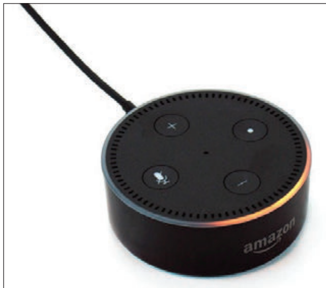
Figure 9-48 The orange light indicates the Echo Dot is on but not connected to a Wi-Fi network
