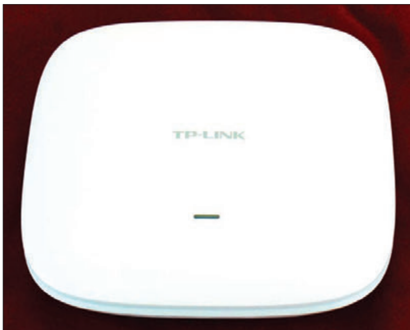
Figure 8-21 A ceiling-mount wireless access point by TP-Link
