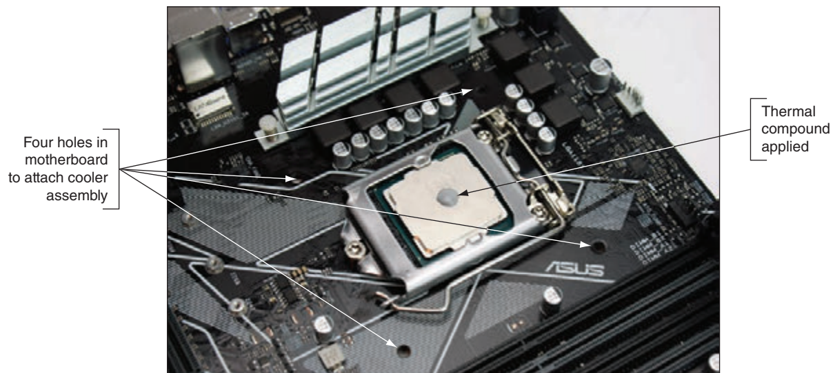
Figure 3-15 If the cooler does not have preapplied thermal compound, apply it on top of the processor
