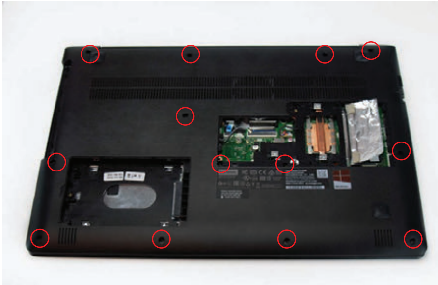
Figure 2-43 The bottom of a laptop with the hard drive, memory, Mini PCI Express card, and optical drive removed
