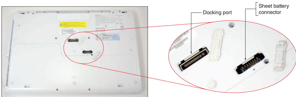
Figure 1-64 The docking port and sheet battery connector on the bottom of a laptop
