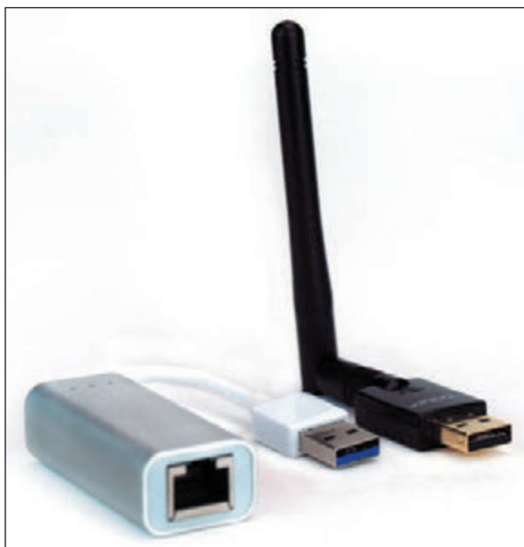
Figure 7-27 USB devices provide wired and wireless network connections
