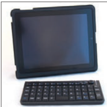
Figure 9-31 An iPad and a wireless keyboard can connect using Bluetooth
