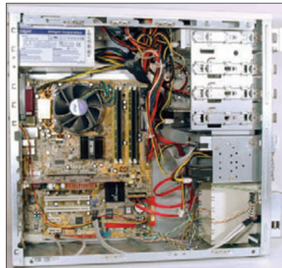
Figure 4-23 Use cable ties to hold cables out of the way of fans and airflow
