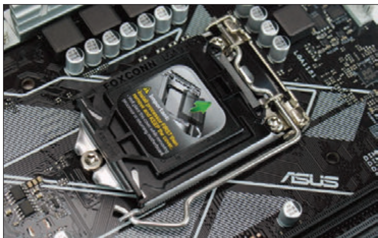
Figure 3-8 The Intel LGA1151 socket with a protective cover in place
