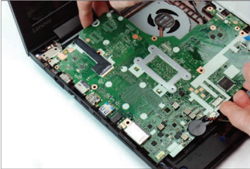
Figure 2-45 Detach the system board from jacks on the left side of the case and then lift the system board up and out of the case
