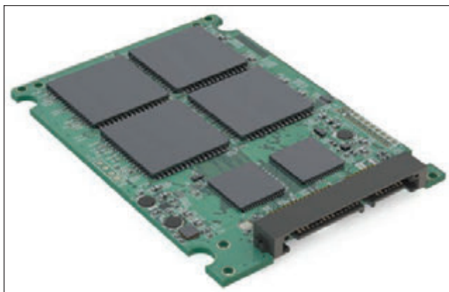
Figure 5-4 A circuit board with NAND memory inside an SSD
