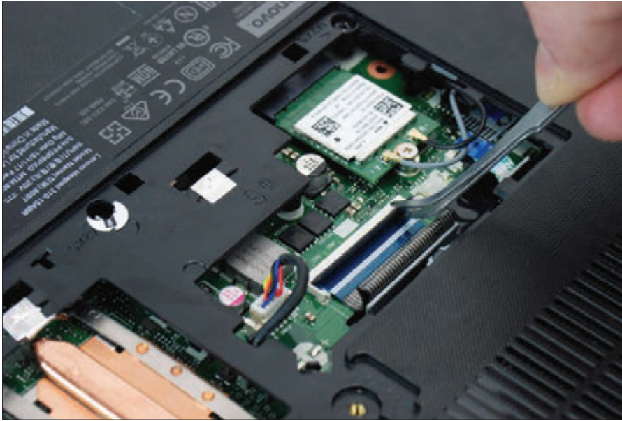
Figure 1-76 To disconnect a ZIF connector, first lift up on the locking flap to release the latch, and then remove the cable using the pull tab, which is blue on this laptop
