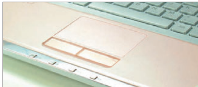
Figure 1-62 The touch pad is the most common pointing device on a notebook
