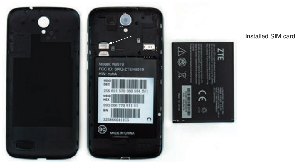
Figure 7-7 A SIM card contains proof that your device can use a cellular network
