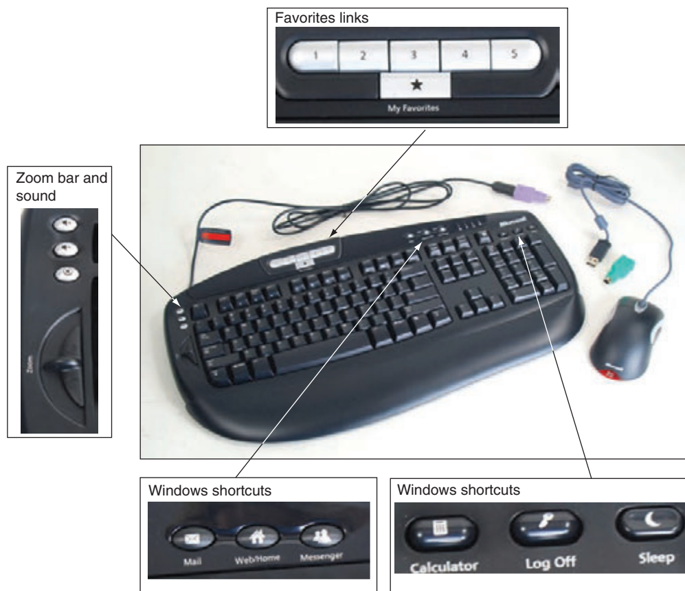
Figure 6-16 The mouse and keyboard require drivers to use the extra buttons and zoom bar
