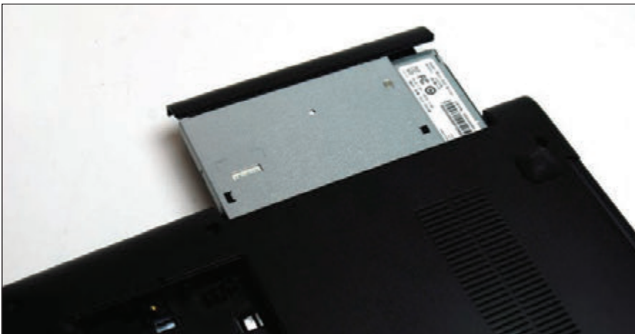
Figure 1-83 Slide the optical drive out of the case after removing the screw securing the optical drive to the laptop
