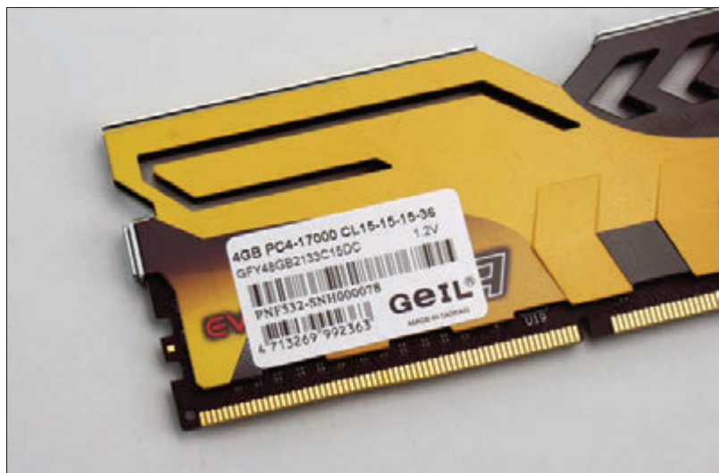
Figure 3-40 Use the label on this DIMM to identify its features
