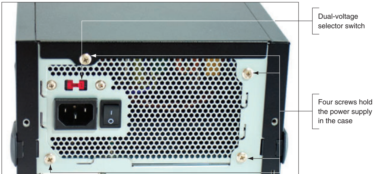
Figure 1-19 The dual-voltage selector switch sets the input voltage to the power supply
