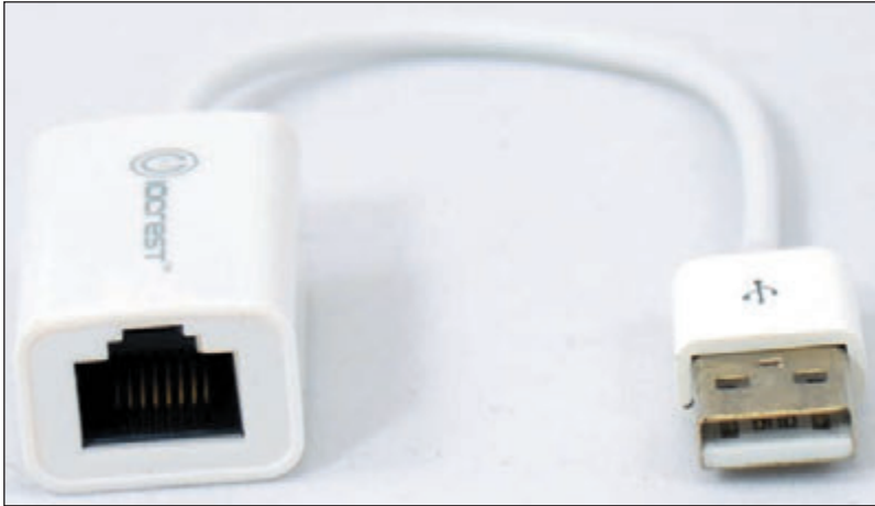
Figure 1-58 A USB to RJ-45 dongle provides a network port to connect to a wired network
