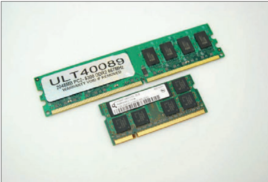
Figure 1-80 A DIMM used in desktops compared with a SO-DIMM used in laptop computers
