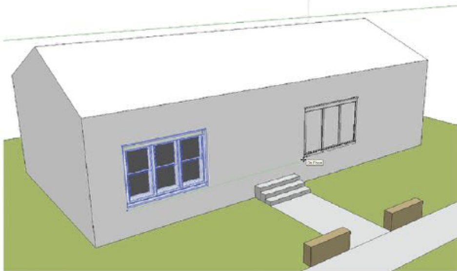
Fig. 6-37: Building components can be scaled and adjusted like regular components while fixed to a face.
