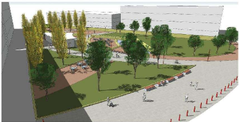
Fig. 16-14: The final model view, with components copied into blocks to create a quick 3D detailed site model.
