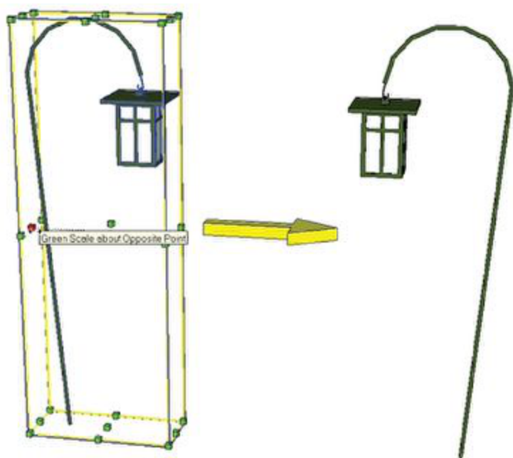
Fig. 8-4: Mirrored and inverted component.
