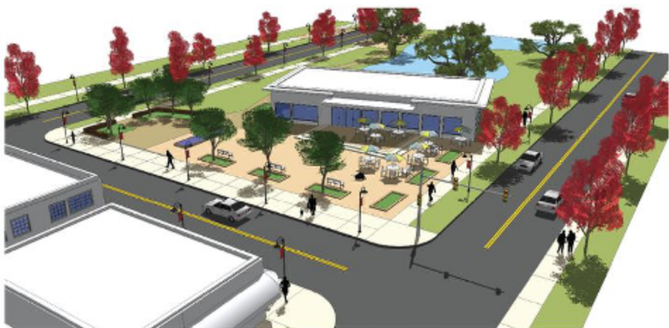
Fig. 6-43: Component details are added to the Flatwork Base. Components were downloaded from Google 3D Warehouse Bonus Pack for SketchUp 7 and from www.formfonts.com .
