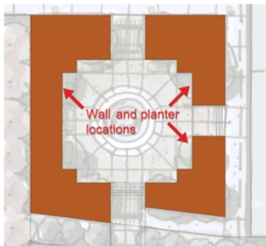
Fig. 7-29: Offset the planter area faces to create edges for the wall.
