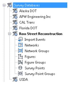
The survey database can be created either locally, or on a network, and you import survey data collected from a number of sources. Survey observation data that resides in the survey database may be recreated in different drawings with different coordinate systems. This is especially useful when you need to produce drawings that represent grid coordinates, as well as drawings that represent ground coordinates from a common survey database.
