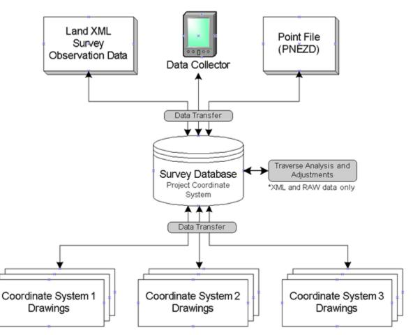
The survey data can be accessed through multiple drawings and can affect other objects, such as points and surfaces. For example, when you change a prism height or a backsight angle, associated point data automatically updates.
