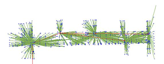
Survey networks provide a repository for the data collected in land development projects. Each project phase, or location, can be represented by a network in the database. Once the network is created, survey data can be transferred to the database from total station and GPS data files.
