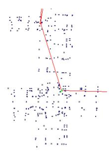
The survey network is an object that visually represents the data in your survey. It is used for editing and analyzing survey data. After the survey has been analyzed for errors and adjusted, the survey network is removed from the drawing. The adjusted points and the figures are then inserted to the drawing from the survey database.
