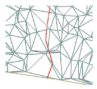
When you use the 3D polyline to create a standard breakline, the elevations at each of the line's vertices are added to the surface. When you rebuild the surface, no triangles cross the breakline.
