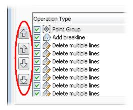
When you create and edit a surface, you can perform many different types of operations to add data and edit surfaces. The order and inclusion of these operations could produce undesired results. The Operation Type list makes it easy to track the operations you perform on a surface, undo or redo the operations, and change the order in which operations are executed.
