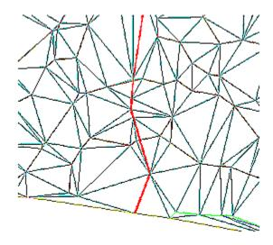
Notice how the polyline crosses the triangles that describe the surface in the illustration on the left. The illustration on the right shows the same polyline made into a breakline. Notice how the surface triangles follow the breakline, increasing the accuracy of elevation calculations at this part of the surface.
