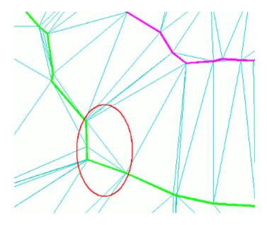
With the Swap Edge command, you can change the direction of triangle lines to improve the accuracy of the surface. In the following illustration, two triangle edges that connected the same contour were edited. In the original version of the surface, the contours were oriented from upper left to lower right. In the current version, they are oriented from lower left to upper right.
