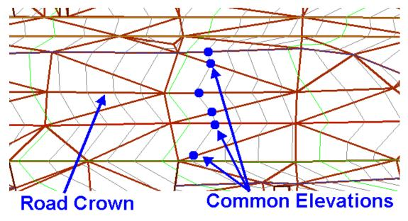
You can create two types of surfaces. Regular surfaces are used to model existing and proposed terrain. You use volume surfaces to calculate site volumes by referencing an existing and a proposed surface.
