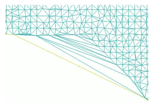
The following illustration shows the same area of the surface after you delete the triangles. The surface border now coincides with the limit of the point data.
