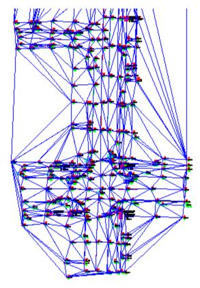
This following illustration shows the surface with the maximum triangle length set to 75' (20 m).
