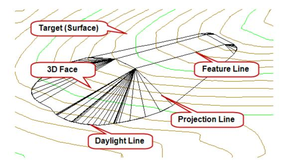
From the 3D angle, you can see the rectangular building pad that is used as the footprint and you can also see the daylight line (sometimes referred to as a catch line) where the projection lines intersect the target surface in this fill situation.
