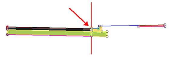
The lane subassembly in the cul-de-sac assembly has a fixed width. The width of the lane subassembly and the elevation of the inside crown is overridden by assigning the optional alignment and profile target to the centerline alignment and profile of the cul-de-sac alignment. This essentially stretches the lane back to the centerline alignment and elevation in the cul-de-sac. The following illustration shows the completed cul-de-sac without targets assigned to the lane subassembly.
