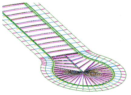
Corridor surfaces are useful for design and construction tasks. You can use corridor surfaces to calculate earth cut and fill quantities, label spot elevations and slopes, and generate construction staking data.
