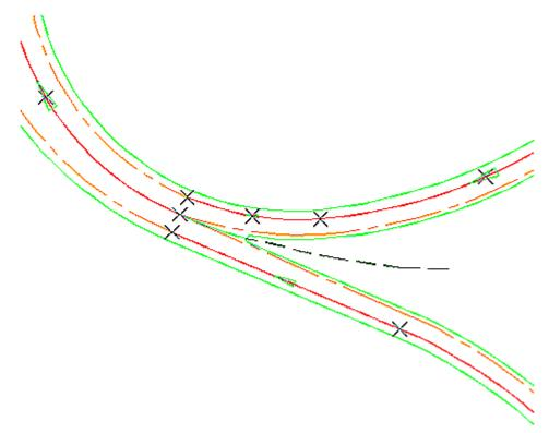
The illustration shows the same alignments after a corridor is created. Different assemblies are applied along the alignments to create a single corridor with lanes and ditches that merge together seamlessly. Each alignment is associated with the corridor model by using a different baseline entry in the corridor properties.
