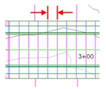
The assembly insertion frequency is not related to the increment at which cross sections can be created, and can be changed when you modify the properties of the corridor.
