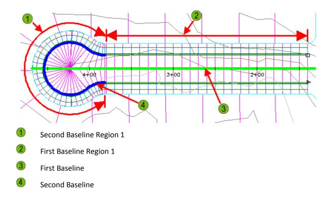
The assembly that you process along the first baseline represents a symmetrical cross section up to the right-of-way locations. The assembly you process along the second baseline for the cul-de-sac is an asymmetrical cross section with the baseline at the edge of pavement location. The assembly baseline is indicated by the arrow in the following illustration.
