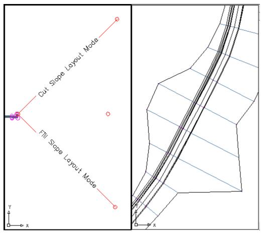
The image on the left shows the subassembly as part of the right side of an assembly, attached to a curb and gutter. The image on the right shows the result of the logic built into the subassembly when it is used in a corridor model. The width of the slope adjusts to account for changes in the terrain.
