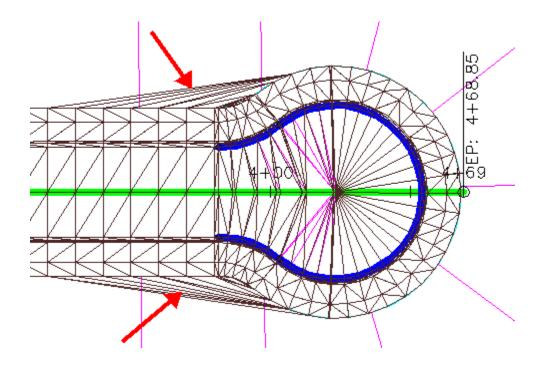
The following illustration shows the same corridor top surface with the boundary defined. In this case, the triangulation lines are contained by the boundary of the corridor surface.
