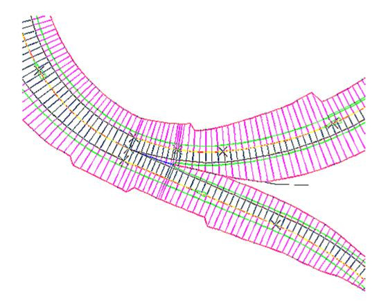
The illustration shows a transition between regions in a corridor. The upper region of the corridor uses an assembly with a plain shoulder. The lower region uses a similar assembly that has a curb and gutter instead of the paved shoulder.
