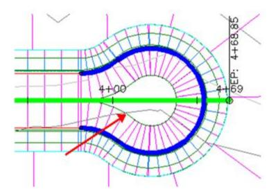
When you assign targets to the lane subassembly on the asymmetrical assembly for the second corridor region, the lane stretches back to the centerline alignment location and elevation. This is shown in the following illustration.
