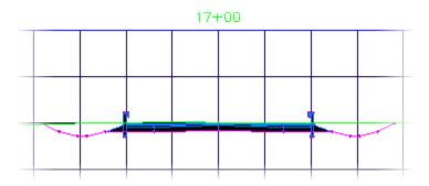
Sample lines are required to calculate quantities and to create section views that display section data. Sample lines are attached to an alignment, as shown in the following illustration.
