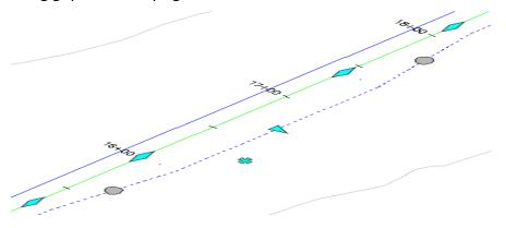
An engineer is planning a two-lane road with parallel lanes located 12' from the left and right sides of the centerline. To accomplish this you would create two offset alignments.
