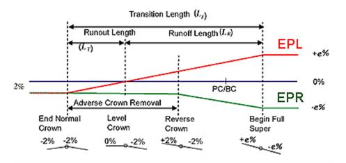
The following image shows an example of an alignment where the superelevation stations overlap. You can manually adjust the superelevation by adding, removing, and changing the location of superelevation critical points.
