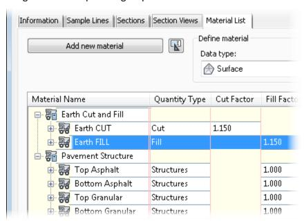
Quantity reports are created from a sample line group and can be inserted in a drawing as a table, or extracted to an external file. After a quantity report is created, if the corridor model changes, the section data attached to the sample lines also updates. When the section data attached to the sample lines updates, the quantity table in the drawing also updates. This
