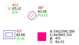
The Civil 3D point object consists of a marker and a label. The display of the marker is controlled with a point style. In this illustration, you can see how different point styles can be used to show different types of points. The display of the label is controlled with a point label style. Different label styles can be used to show specific point data.
