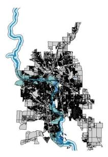
The following illustration overlays two layers, a flood zone, and a parcel layer, in order to determine where the two intersect. The intersected parcels layer becomes a new layer, which can be styled and used for additional analysis.
